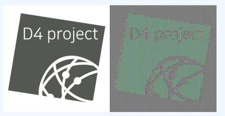
Figure: Image encrypted with AES-ECB
